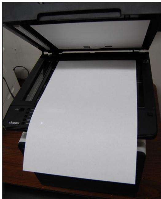
A unique feature of the M402dn lets users copy an 11"-x-17" page by placing it on the platen and pressing the A3/11 x 17 START button (rather than the start key, which is covered by the page) to initiate the copy.
