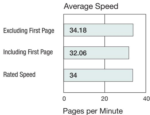
Print speed is tested using BLI's Monochrome Test Original with 6% page coverage. The test page is printed in a quantity equal to double the vendor's rated print speed for the device in each mode tested (e.g., if the vendor's rated print speed is 20 ppm, 40 pages are printed). The unit's print speeds were tested using the PCL driver.
